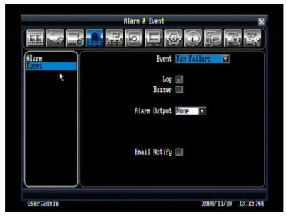
Figure 5.13 (Alarm & Event Menu – Event-Fan Failure)
